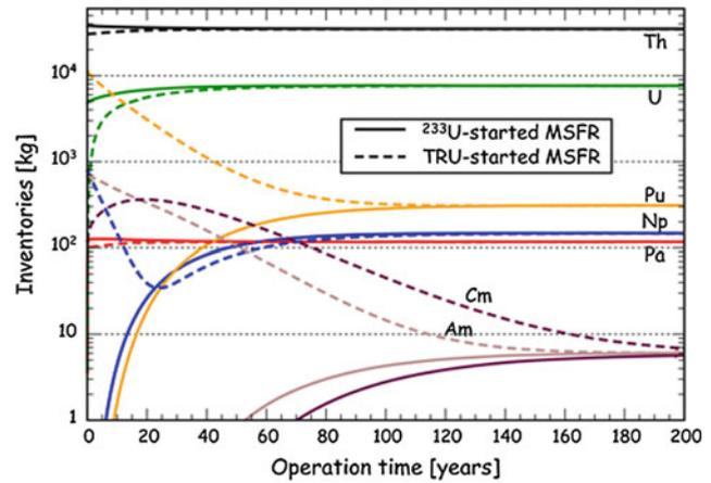
**Fig. 5** Time evolution up to equilibrium of the heavy nuclei inventory for the  $^{233}\text{U}$ -started MSFR (solid lines) and for the TRU-started MSFR (dashed lines). Operation time is given in equivalent full power years (EFPY) [14]
