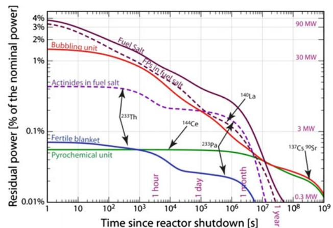
**Fig. 7** Residual heat in the different radioactive fluids of the MSFR, after the total fission shut-down of the reactor previously under steady-state conditions [12, 17]
