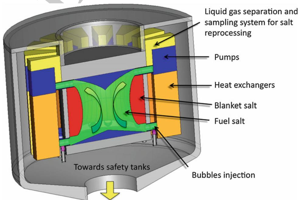
the fuel salt into tanks located under the reactor and where a passive cooling and adequate reactivity margin can be implemented.
