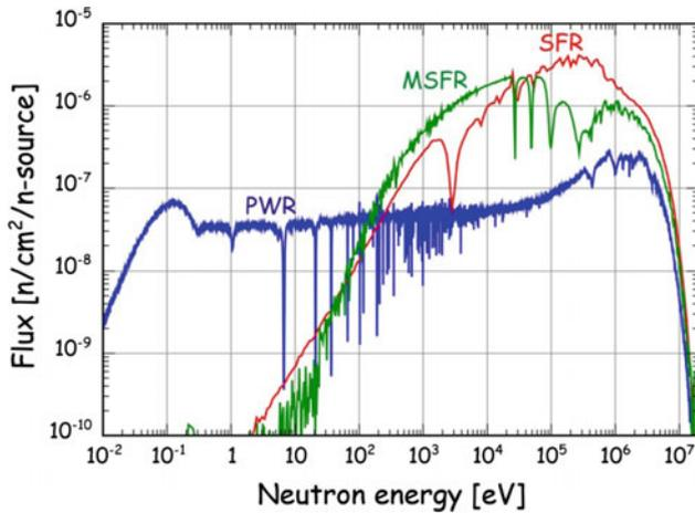
**Fig. 8** Fast neutron spectra of the reference MSFR (green curve) and of a sodium-cooled fast neutron reactor (SFR, red curve) compared with the thermalized spectrum of a pressurized water reactor (PWR, blue curve) [14]
