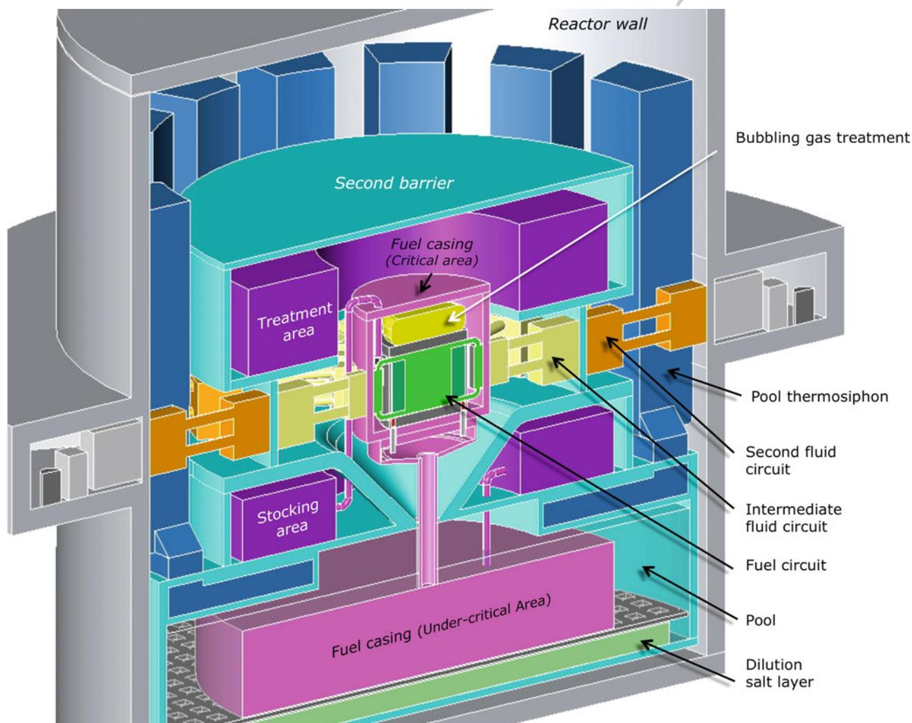
**Fig. 2** Illustration of the main functions associated with the MSFR operation. In the middle is the *green* fuel salt circuit surrounded by a *pink* envelope representing the first confinement barrier. The *cyan* envelope represents the second barrier, including storing and chemical
