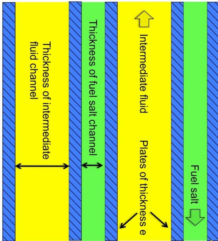
Two kind of intermediate fluid considered in this study: liquid metal or fluoride salt
