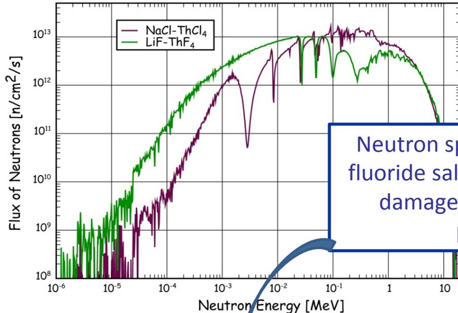
Neutron spectrum less fast with fluoride salt = reduced irradiation damages (both DPA and He production)
