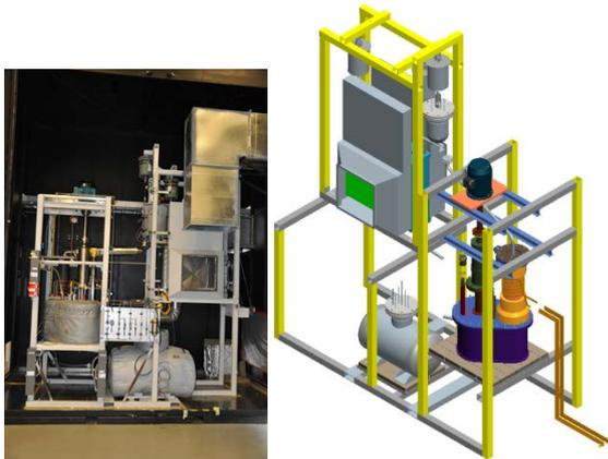
Fig. 8 ORNL Liquid Salt Test Loop (as design drawing (left) and as constructed (right))
