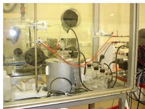
Figure 5: Glove box dedicated to ThF<sub>4</sub>-based molten salts studies, particularly electrochemical steps of the reprocessing (CNRS, France)
