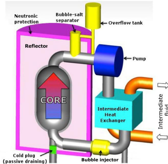
FIG. 3. Schematic view of the MSFR demonstrator with one of the 6 external loops
