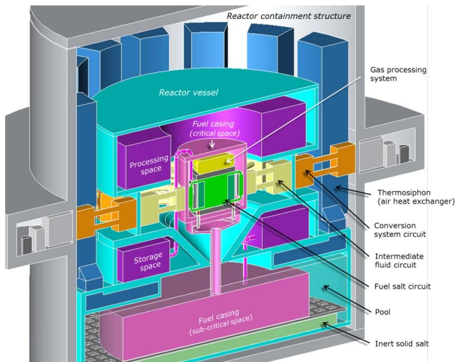
Fig 2. Layout of the MSFR reactor systems showing the 3 containment barriers
