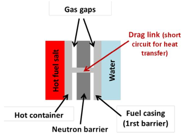
Fig 6. Example of transversal structure of the draining tank walls (not to scale)
