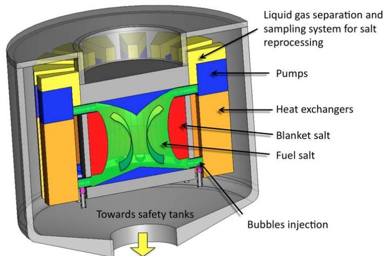
Fig.1. Schematic conceptual MSFR design (fuel salt in green, fertile blanket salt in red)
