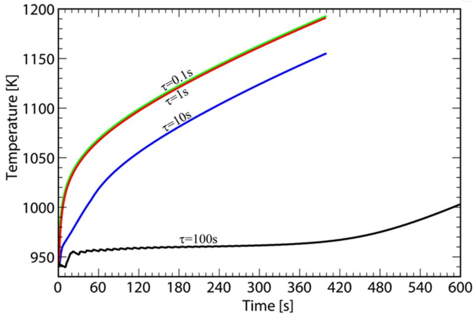
Fig 4. Mean fuel salt temperature after an exponential loss of cooling with a characteristic time of 1s, 10s and 100s ( $C_p$  constant here)
