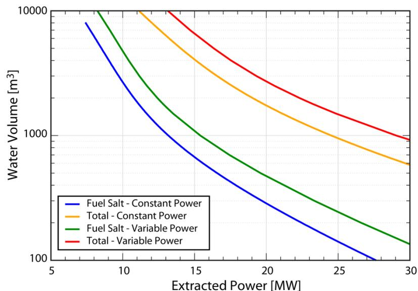
Fig 9. Water mass (in tons) necessary to absorb the residual heat by heating from 30°C to 100°C with the heat extraction given in abscissa (MW)
