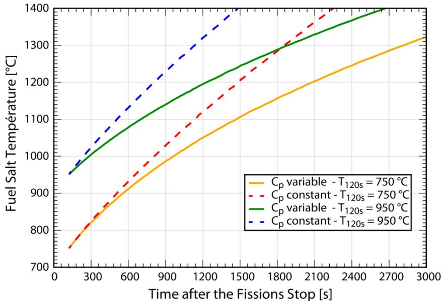
Fig 5. Adiabatic heating of the fuel salt by the decay heat
