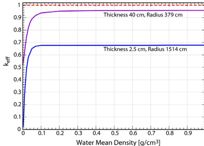
Fig 8. Draining tank criticality as a function of the water density, while considering one single salt layer
