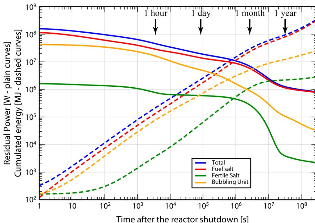
Fig 3. Evolution of the decay power (solid curves) and the corresponding cumulated energy (dashed curves) in the fuel salt, the fertile salt and the bubbling reprocessing unit after the reactor shutdown
