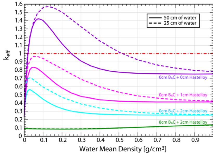
Fig 7. Draining tank criticality as a function of the water density, while considering 18 salt layers separated by water
