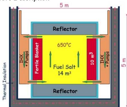
Fig.2. To scale vertical representation of the TMSR, including pumps and heat exchangers (IHX)
