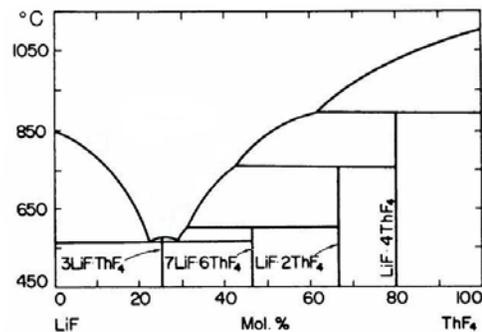
Fig. 3. LiF -  $\text{ThF}_4$  phase diagram
