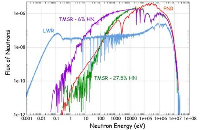
Fig.5. Neutron spectrum of two TMSR configurations (6% and 27.5% of heavy nuclei in the salt) compared to the neutron spectrum in a Light Water cooled Reactor (LWR) and in a Fast Neutron Reactor (FNR)
