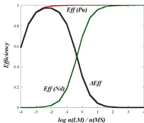
Fig. 1: Extraction efficiency of Pu (in red) and Nd (in green) as a function of the mole ratio  $n(LM)/n(MS)$ . The black curve gives the efficiency difference between Pu and Nd. Liquid metal is metallic Bi containing metallic Th ( $x(Th)=10^{-3}mol\%=solubility$ ). Molten salt:  $LiF-ThF_4$  (77-23mol%) at  $700^\circ C$
