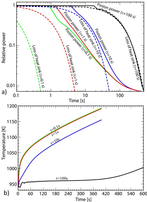
Fig. 5. a) Evolution of the fission power and the extracted heat relative to nominal power as a function of the time since the beginning of the transient; b) Evolution of the mean fuel salt temperature in the core during the transient. Four transients considered: with an exponential heat sink loss with  $\tau=0.1s$  (green curves), 1s (red curves), 10s (blue curves) and 100s (black curves).
