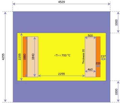
Fig. 2. MSFR configuration of the EVOL neutronic Benchmark (dimensions given in mm) with fuel salt (yellow), the fertile salt (pink) the  $\text{B}_4\text{C}$  protection (orange) and the reflectors and the 20mm thick walls in Ni-based alloy (blue).
