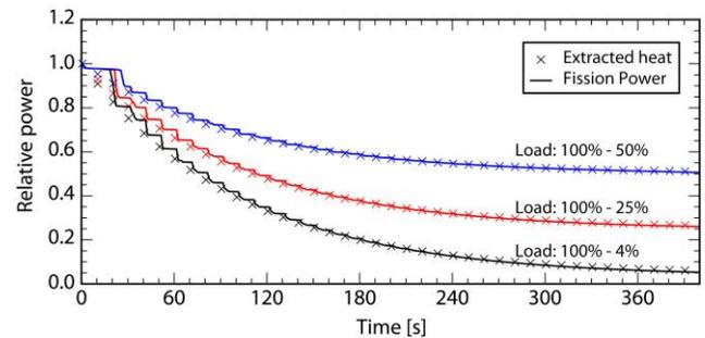
Fig. 4. Fission power with the extracted heat relative to nominal power for different load followings: 100% - 50%, 100% - 25% and 100% - 4%.
