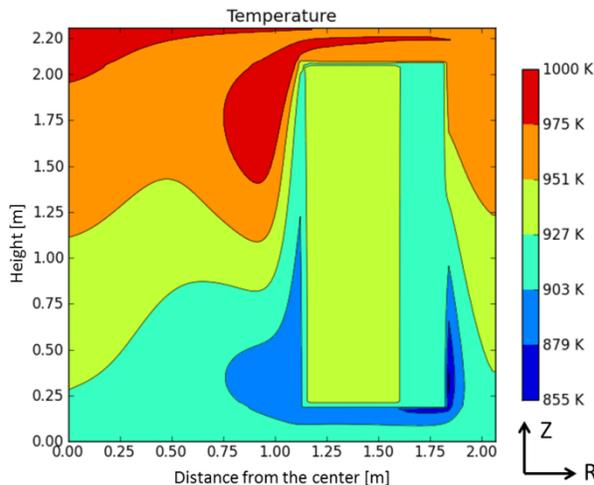
Fig. 3. Temperature distribution in the half MSFR core model calculated with COUPLE. The fuel salt circulates upwards in the core (on the left) and downwards in the heat exchanger (on the right). In between is the fertile blanket with the neutronic protection.
