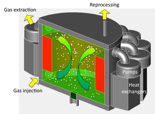
Fig. 1. A simplified schematic of the MSFR system including the fertile blanket (red) and the fuel salt (transparent green) circulating in the core, pumps and heat exchangers.
