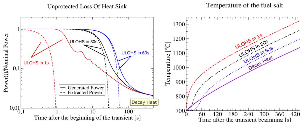
**Figure 4. On the left: Transients after an Unprotected Loss Of Heat Sink in 1s (in red), 30s (in black) and 60s (in blue): the extracted power (dashed curves) and the power in the core (solid curves) including the fissions and the decay heat. On the right: Temperature of the fuel salt only due to the decay heat without fissions (violet solid curve), for unprotected loss of heat sink in 1s (red dashed curve), 30s (black dotdash curve) and 60s (blue dotted curve).**
