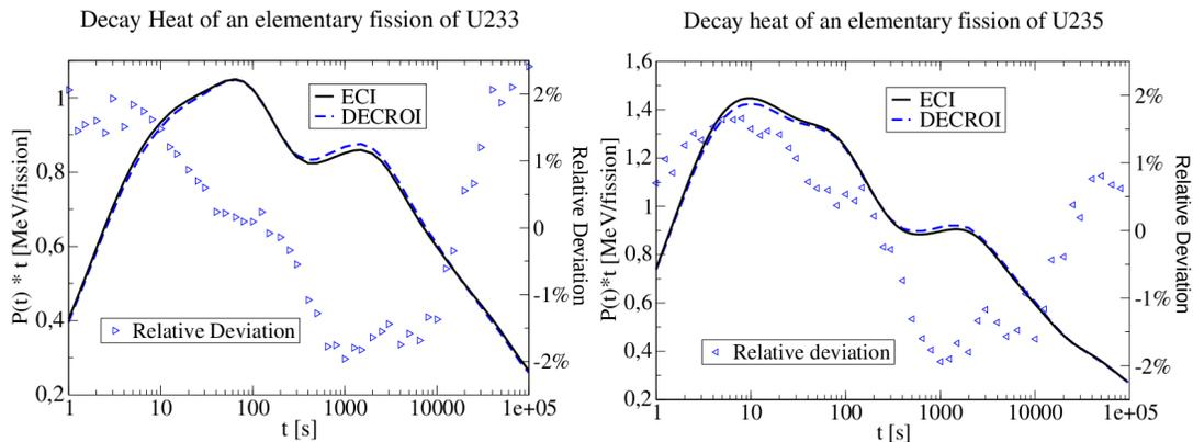
**Figure 2. Comparison of ECI to DECROI calculations on the decay heat of an elementary fission of  $^{233}\text{U}$  (left) and  $^{235}\text{U}$  (right)**
