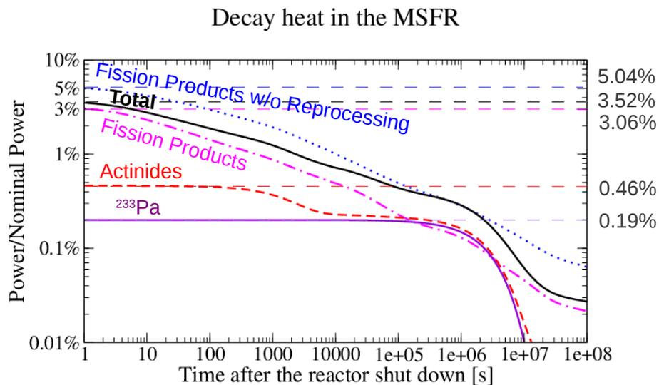
**Figure 3. Residual heat in the MSFR, total: including fission products and actinides, fission products accumulated in the core, actinides and the decay heat of all fission products of  $^{233}\text{U}$  fissions, neglecting all nuclear reactions after the fission and the reprocessing systems.**
