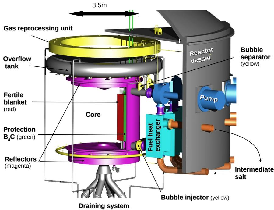
**Figure 1. View of the MSFR systems in contact with the fuel salt, done by A3I**
