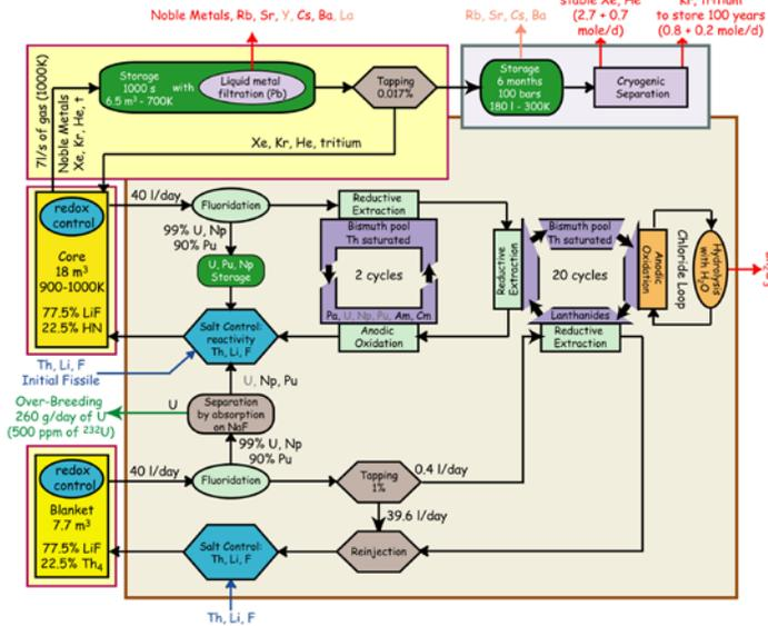
Fig. 3: Overall scheme of the fuel salt management including the online gaseous extraction (top) and the offline reprocessing unit (bottom) – The yellow boxes surrounded by a red line are enclosed within the reactor vessel
