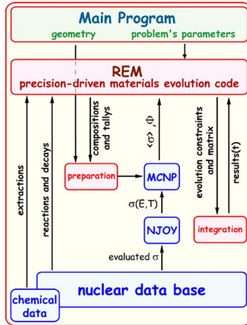
Fig. 4: Coupling scheme of the MCNP neutron transport code with the in-house materials evolution code REM
