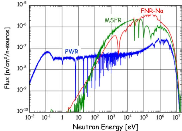
Fig. 2: Fast neutron spectra of the reference MSFR and of a Na-cooled fast neutron reactor (FNR-Na) compared to the thermalized spectrum of a pressurized water reactor (PWR)
