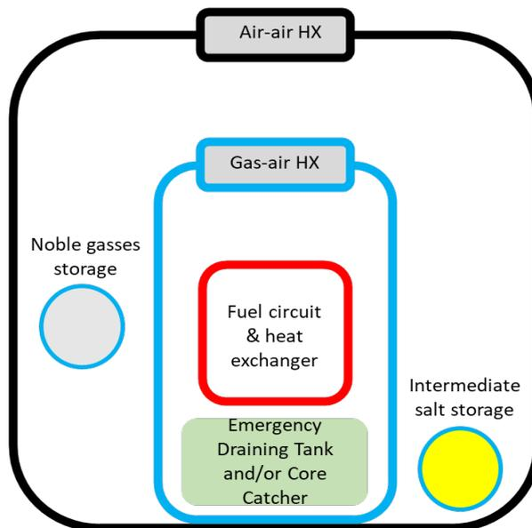
FIG. 4. Schematic representation of the three confinement barriers of the MSFR. The first, in red, is the Core Vessel containing the fuel circuit and the intermediate heat exchanger. The second, in light blue, is the Reactor Casing containing the DHR devices and the draining tanks, including the Core Catcher, and the third, in black, is the Reactor Building containing other radioactive sources.
