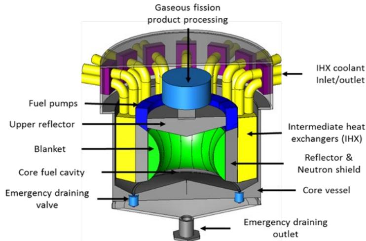
FIG. 2. MSFR fuel circuit components [4], the fuel salt itself being not displayed here.
