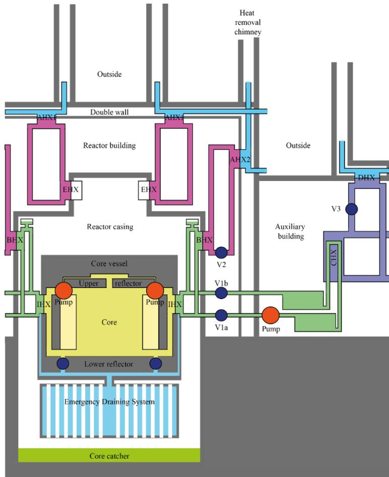
FIG. 3. Components related to the heat extraction in the MSFR system, with the fuel circuit in yellow, the intermediate circuit in green and a part of the energy conversion circuit in purple (from left to right).
