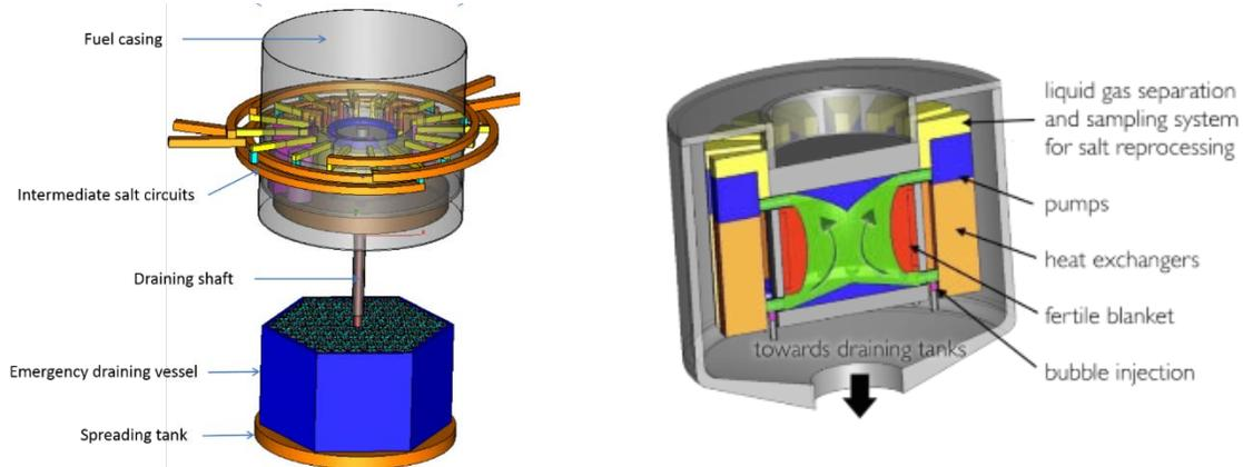
FIG. 1. Schematic view of the MSFR fuel circuit and emergency draining tank (left) and zoom on the fuel circuit (right).
