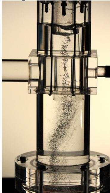
**Figure 20.** Water mock-up of the separator showing the concentration of bubbles in the vortex center and their coalescence. The gas is evacuated at the top and the liquid through the pipe on the left
