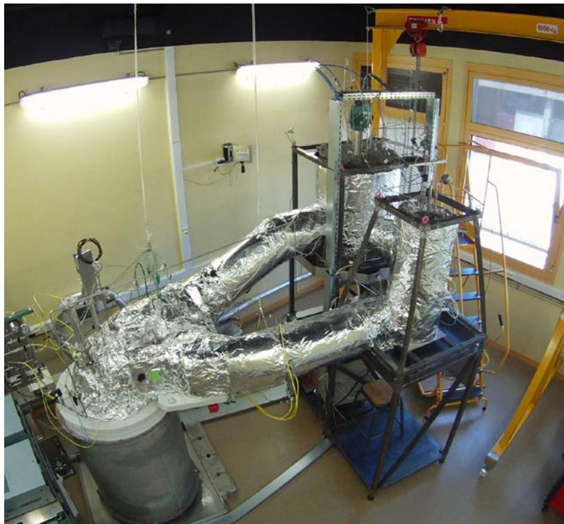
**Figure 19.** Completed loop with its thermal insulation
