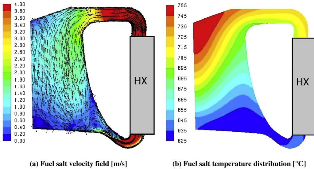
Fig. 5. CFD predictions for the 3D model of Geometry I.
