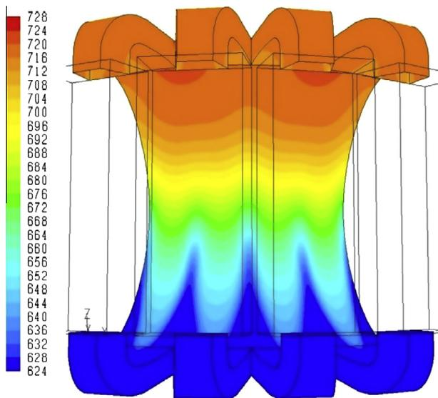
Fig. 7. Temperature [°C] in a symmetry plane of an inlet/outlet and on the walls.
