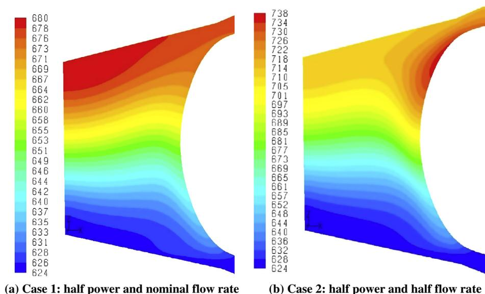
Fig. 8. Temperature distribution [°C] at two different reactor working conditions (Geometry II 3D model).
