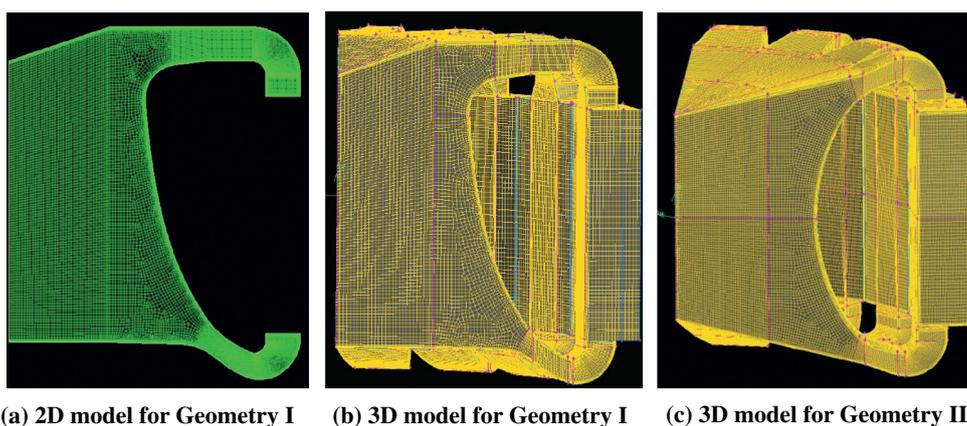
Fig. 3. CFD meshes used in the thermal-hydraulics studies. The HXs shown in the 3D geometry are approximated in the CFD study as a porous medium.
