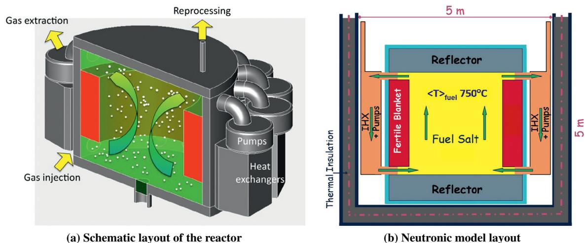
Fig. 1. Molten Salt Fast Reactor (MSFR).
