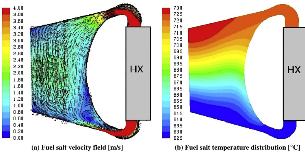
Fig. 6. CFD predictions for the 3D model of Geometry II.
