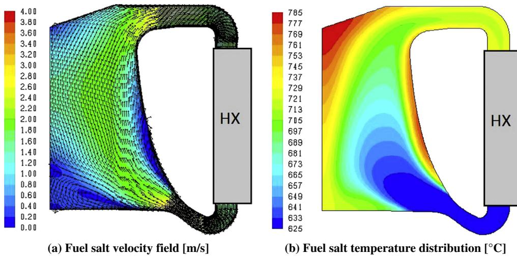
Fig. 4. CFD predictions for the 2D model (radial symmetry) of Geometry I.
