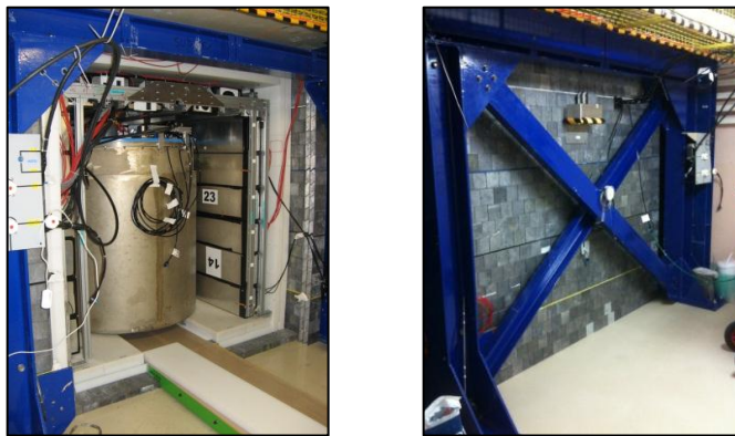
Figure 10: Nucifer shielding surrounding the inner detector (left) and support structure (right).
