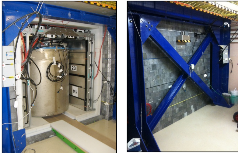
Figure 6: Nucifer shielding surrounding the inner detector (left) and support structure (right).
